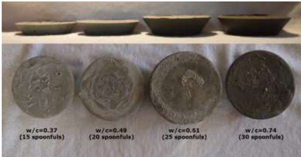
Figure 1. Influence of w/c ratio on the thickness and color of the cement puck
