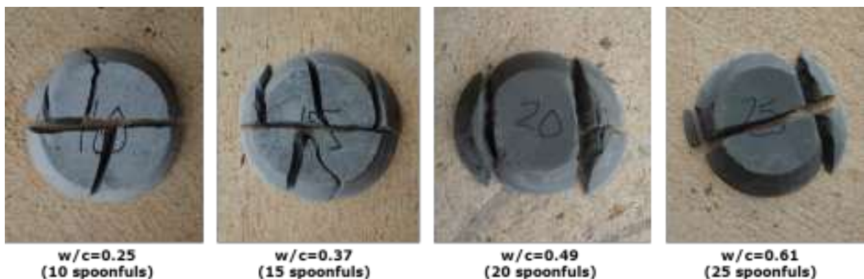
Figure 2. Pucks with different w/c ratios after dropping from a height of at least 15 feet.
