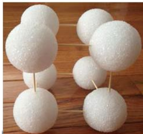
Figure 3: A basic structure, simple cubic, to be built during the student activity portion of this lesson.
